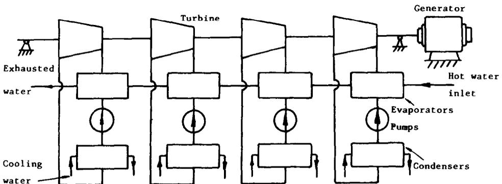
Fig. 8. The schematic of the new multistage cycle equipment.
