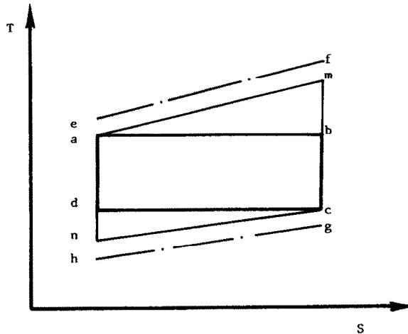
Fig. 1. The Carnot cycle in the  $T$ - $S$  plane.
