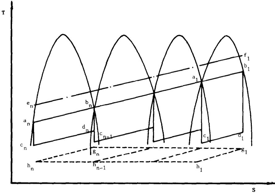
Fig. 7. The  $T$ - $S$  diagram for the new multistage cycle.
