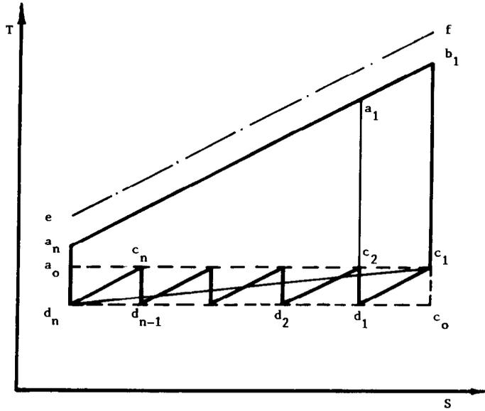
Fig. 5. The new multistage cycle in the  $T$ - $S$  plane.
