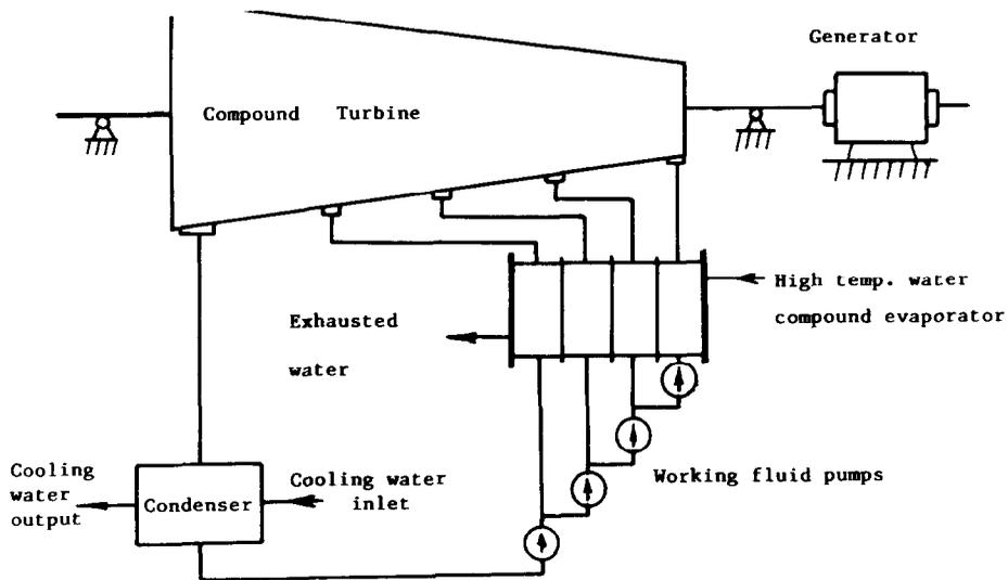
Fig. 9. The schematic of the new compound cycle equipment.
