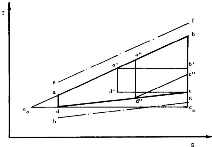
Fig. 4. Comparison of the new cycle with the Carnot and Lorenz cycles.
